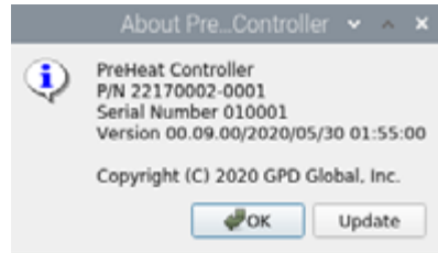
Figure 14: An UPDATE button is present when an update to the control software is available.
